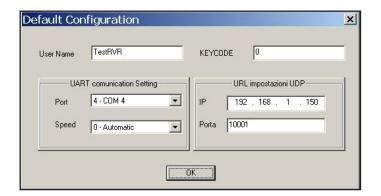
The "UART communication Setting" section allows you to choose the PC serial port used to communicate with the devices and the speed communication from 1200 to 115200. The "Automatic" selection forces the program to groped all connections (1200, 2400, 4800, 9600, 19200, 38400, 57600, 115200) seeking equipment connected.
