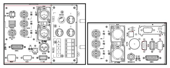
Connect the DB9 connector to the I²C BUS or SERVICE/RDS (depending on model) of /RDS-TEX2HE & /RDS-TEX3HE option to the two BNC ouputs named 19KHZ PILOT OUT (synchronization signal) and SCA1/RDS (RDS signal) always present in the back of the machine itself. If the connecting device is different, identify an equivalent.
