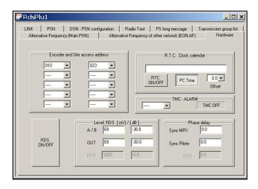
The Address section allows you to assign an identification number of the position in which it will be installed (1-1023) and an identification number of the equipment itself (1-63). This allows to the RDS to recognize only the messages for all and those addressed to him personally. If a device is configured as a Site=9 and equipment=5 it will be recognized itslef on 4 addresses.
