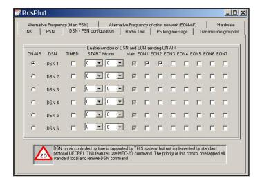
The third example shows an equipment that divides the day in four parts and each part using a different DNS and then in every day section will send a different Radio Texts, and eventually show data with different PSN.
