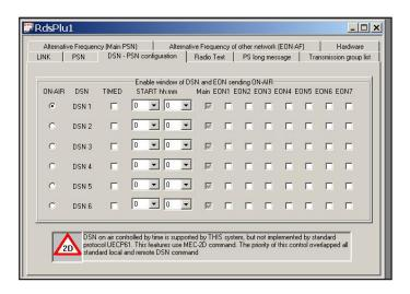
The user that owns an associated network with the other 2 will enable 2 EON as in the example in the following and leave all time controls disabled.
