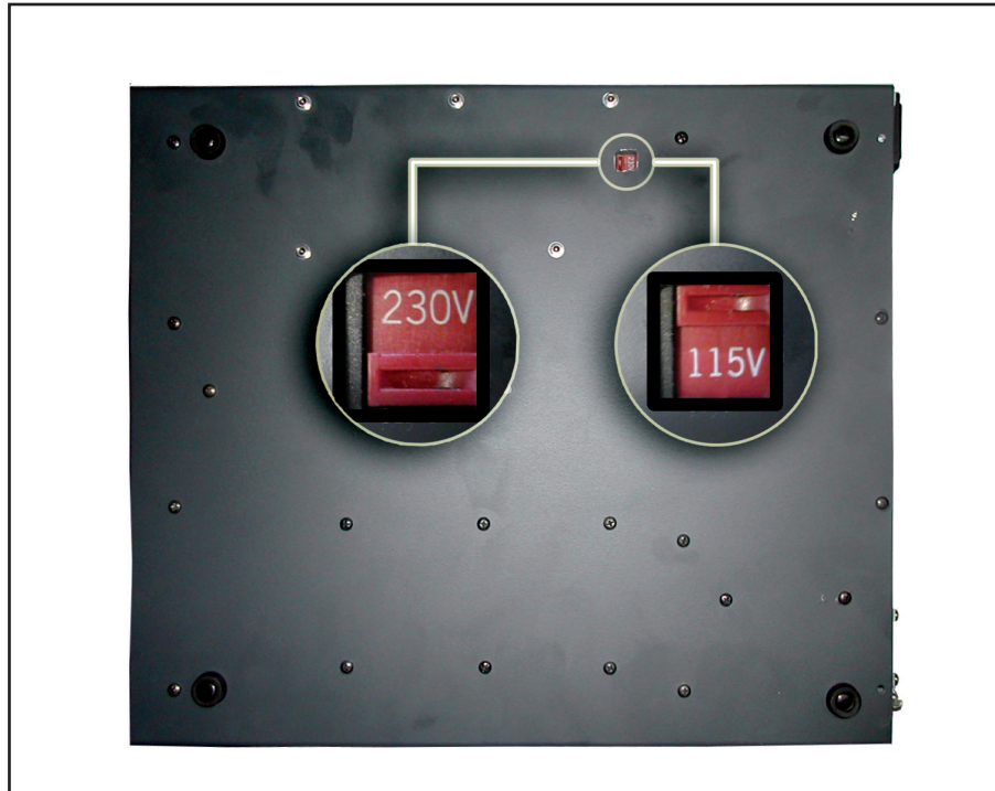
Figure 5.1: switch to change the voltage on the underside URPT / MIC
