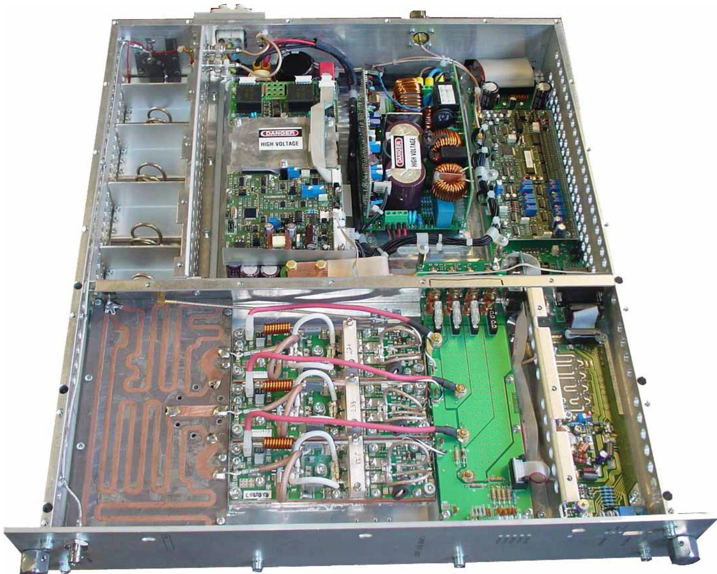
Figure 4-3 Internal view of RF sub-amplifier module
