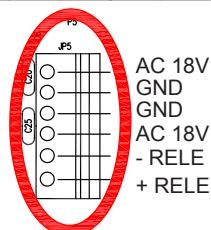
Power supply pinout
