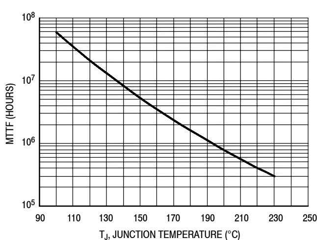
This above graph displays calculated MTTF in hours when the device is operated at  $V_{DD} = 50 \text{ Vdc}$ ,  $P_{out} = 1000 \text{ W CW}$ , and  $\eta_D = 72\%$ .
