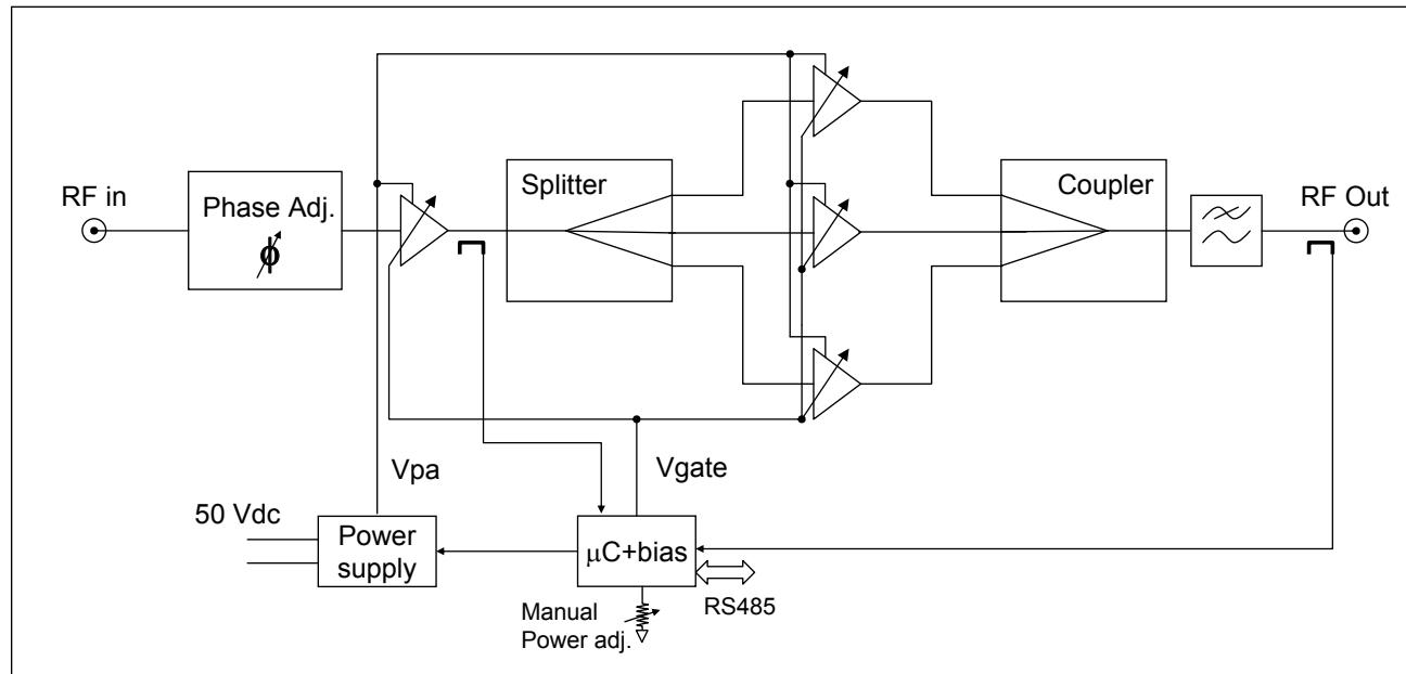
Figure 4-2 Block diagram of RF sub-amplifier module
