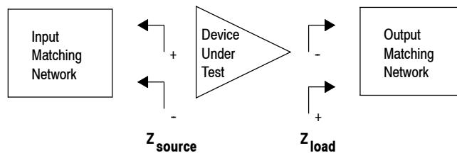
Figure 15. Series Equivalent Source and Load Impedance
