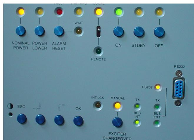
**Note:** the exchange of the exciter and the relative cursor are available only if the logic of exchange is set to manual and the yellow LED is lit.
