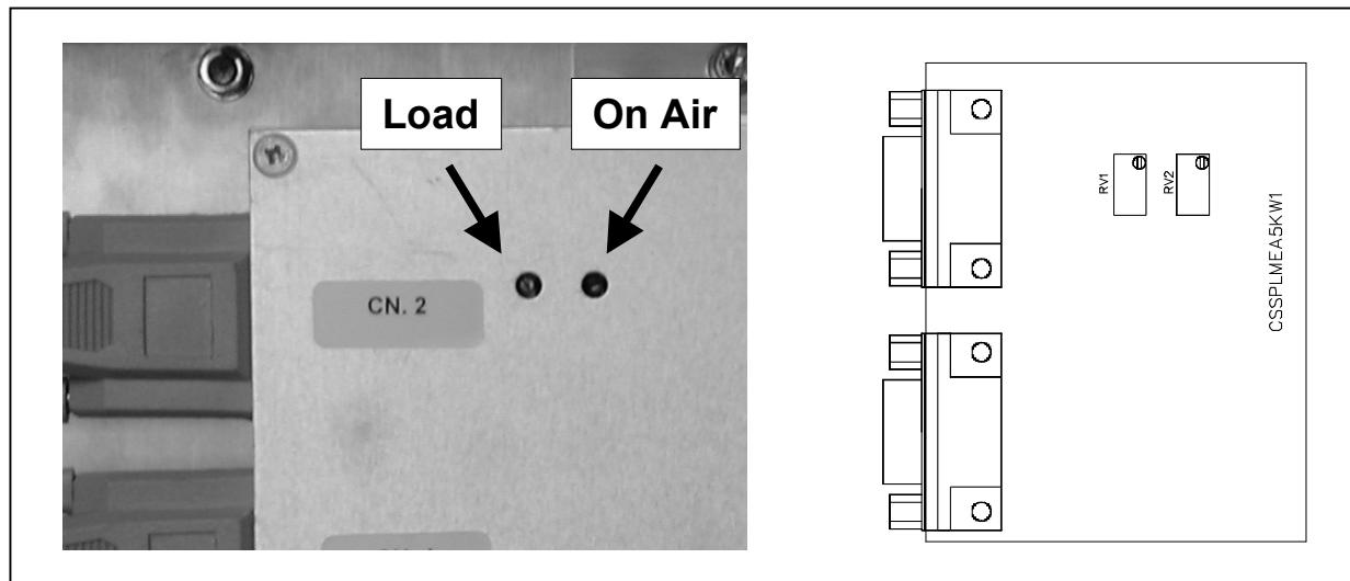
On the circuits of power measure of the exciters there are two compensators to maximize the directive and minimize the operation error measure of the frequency of operation.
