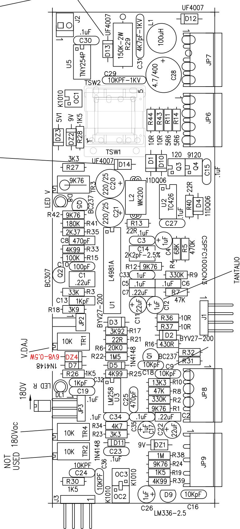
NOTA: TR3 VIENE SOSTITUITO CON UNA RES. DA 9K76
