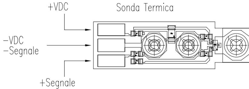
**FIG. 39 -CONNETTORE PER LA MISURA DI P.W.R.**
