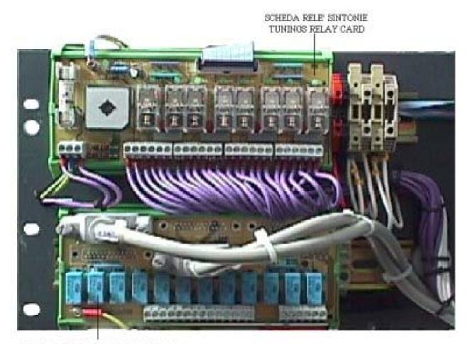
SCHEDA INTERFACCIA TELEMETRIA INTERFACE TELEMETRY CARD
