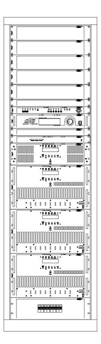
This version of the transmitter is tele-controllable and includes the RDS coder.
