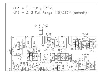
Figure 5.1: Voltage selection jumper on PFC
