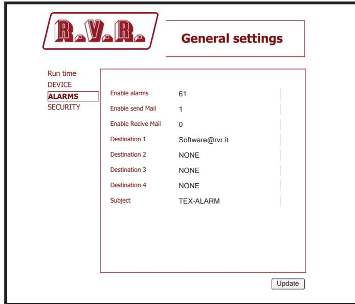
The screenshot shows the 'General settings' page for the 'ALARMS' section. The left sidebar contains a menu with 'Run time', 'DEVICE', 'ALARMS' (highlighted), and 'SECURITY'. The main content area displays the following configuration options:
